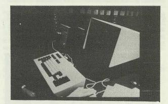
The terminals are of the type that are shown here. It is a 1200 baud terminal. It has a keypad, and a thing called a mouse. On this side you can see a 5-keypad, one key for each of the five fingers. This system extends beyond the concept of just being able to prepare documents easily and distribute them electronically. It allows the more difficult
