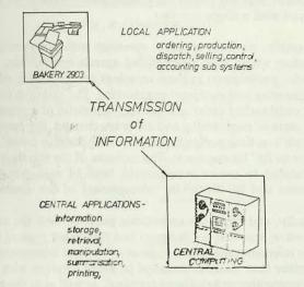
The 2903 minicomputer specified consisted of a 24K word processor, 300 line per minute printer, card reader, operator's console and 20 megabytes of disc (ten of which were fixed and ten demountable). Data entry was to be done by between five and eight direct entry keyboard and screen devices according to the bakery size.
