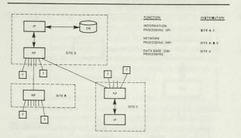
A little later, we added site C over here, which was originally called remote batch or remote job entry; the generic term today seems to be satellite processing. A satellite processor is a smaller version of our host processor up here. Satellite processors generally adopt a subservient role to the host. We have a master/slave or a host/satellite relationship. They do not view each other as co-equals.
