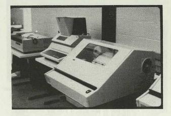
The most recent one that we have announced is called the 'image' printer. The image printer is a fibre optic device.
