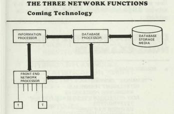
We have seen it already. There is occurring now a second separation of function, wherein the database function will be split off from the host processor and put into a separate machine of its own that is called a database processor. That database processor has already been labelled the back end.
