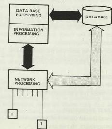
This happened about 1964. General Electric, and Honeywell, and others made what was called a 'separation of function' where the communications activity was pulled out of the host processor and put into a second machine that was very quickly labelled the front end. So the front end network processor then took over the entire communication load, leaving the host processor up there free to do what it was designed for — that is, processing of information.
