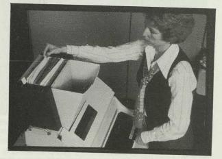
This is another feature which we have on the printer, which is a dual forms feeder. It allows you to put in two forms at the back, one form which would be your heading page of your document and others being subsequent pages. This is all cut paper. It feeds it automatically through the printer and comes up into the stacker which is right at the front. It looks rather like a mincing machine to me.
