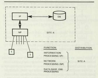
information processing function. When we get our database processor or our back end processor, these pictures will change. So this is our totally centralised network because all three functions exist at the same centralised location.
