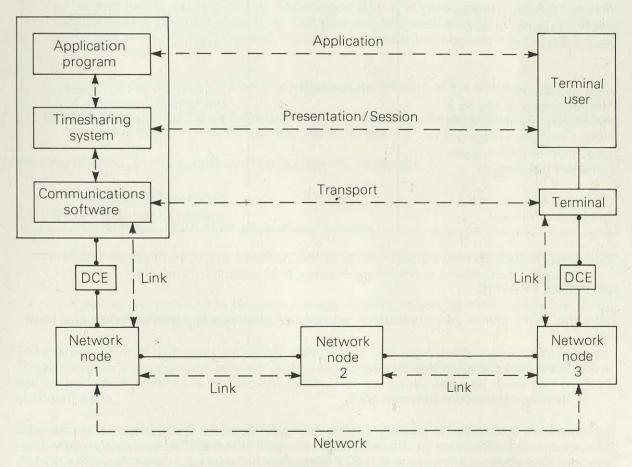
Key: DCE = Data circuit terminating equipment
