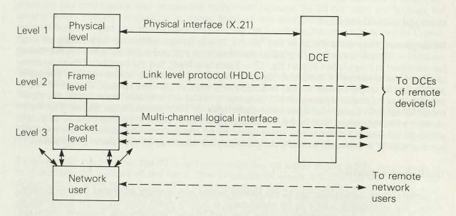
DCE = Data circuit terminating equipment (supplied by the PTT)
