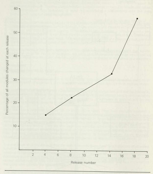
Figure 23 Increasing complexity of the IBM OS/360 structure
