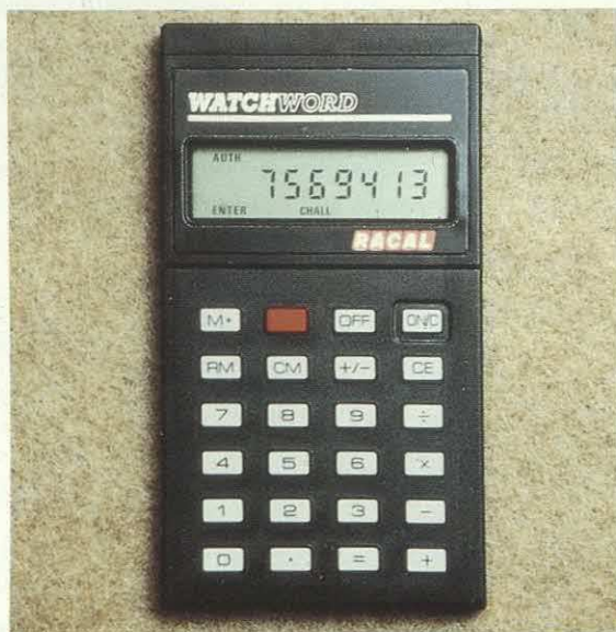
Figure 4 Authenticators are calculator-like devices that can be used with existing terminals
