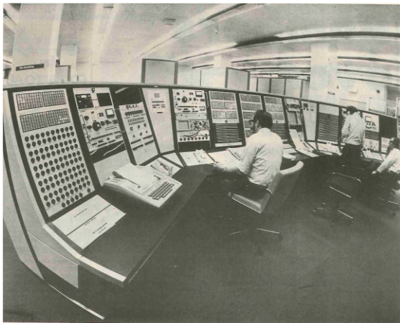
Figure 9 Front End Processing of TOPS messages for the IBM mainframes took place on the Ground Floor Control Room of Blandford House
