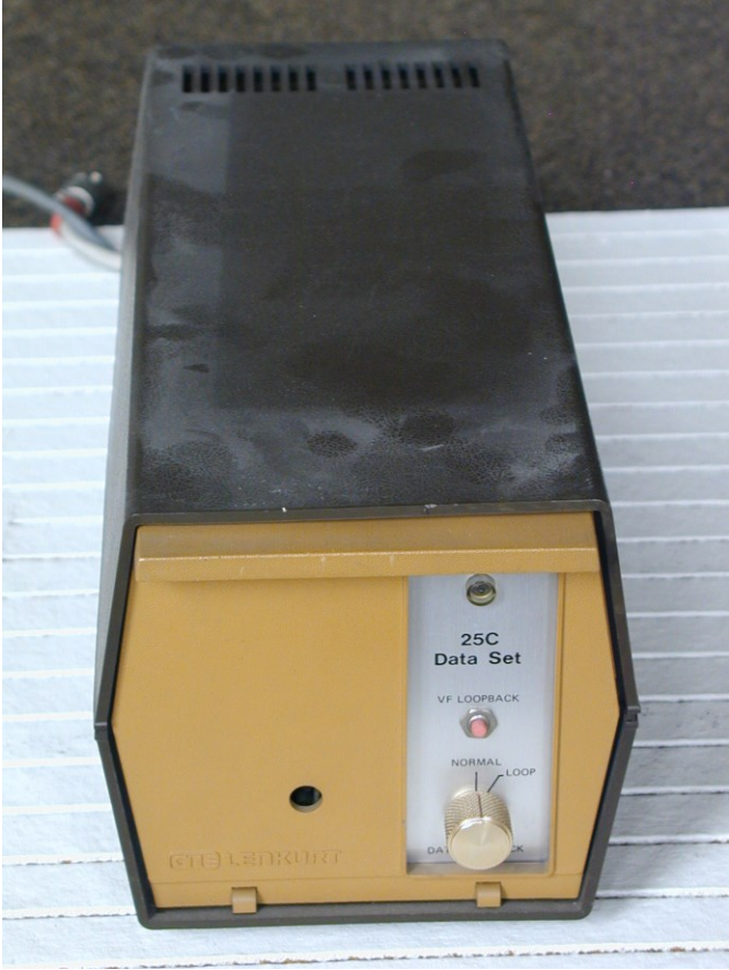
Figure 10 The Lenkurt 25C Modem was one of the technical developments in telecommunications transmission which made adoption of TOPS by BR possible (photo Sam Hallas)
